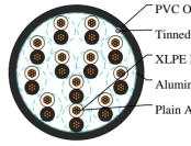
PVC Outer Sheath Tinned Copper Drain Wire XLPE Insulation Aluminium/polyester tape Plain Annealed Copper
